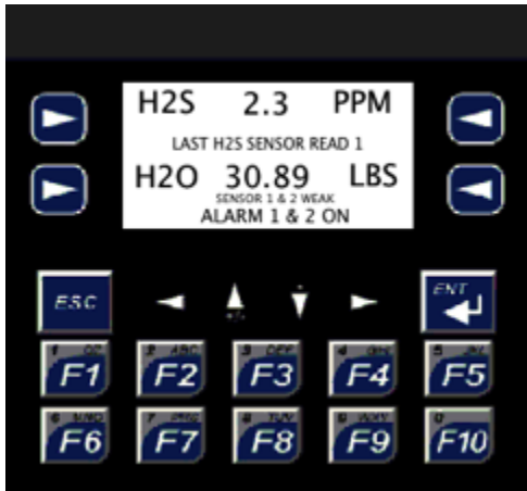
Displays a two channel H 2 S/H 2 O
